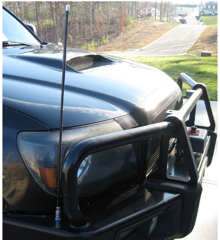
bumper mount (2ft antenna)
