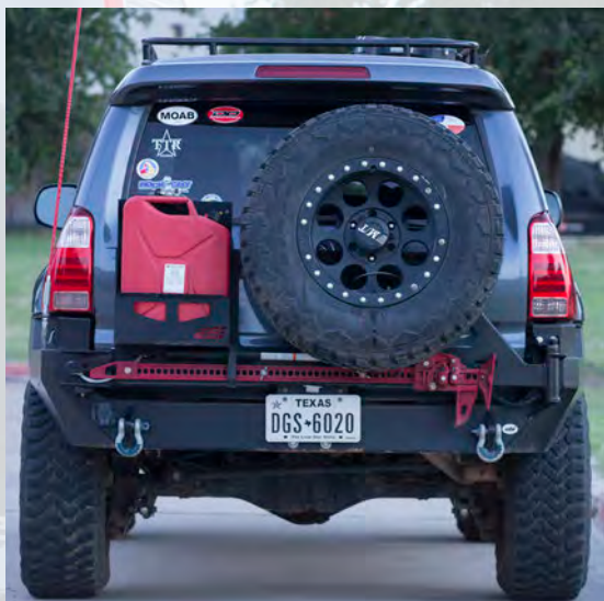
The 4Runner bumper by CBI Offroad Fab is designed to carry fuel, spare tire, and Hi-Lift Jack.
